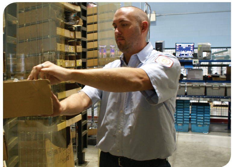
Pick to light technology directs the worker to the exact location of the desired SKU and displays the quantity to pick.
