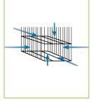
All carriers and shelves are made of wire to provide maximum air flow (all six sides) to help eliminate mold, mildew and spore growth.
