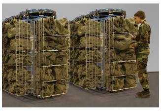
High density ERS provides increased levels of floor space savings, accessibility and productivity. Bags are presented to the operator automatically. During deployment, the system can be designed to be flooded with personnel to provide 100% accessibility.
