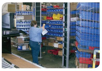
Two Kardex Remstar horizontal carousels to serve as the central distribution point to supply the machine shop and welding workzones.
