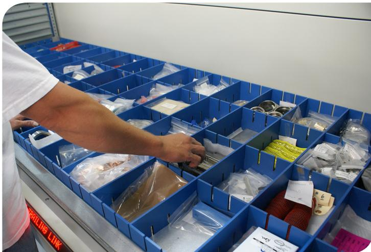
The TIC (transaction information center) located at the front of the access opening uses an alpha numeric display to pinpoint the exact location and quantity for the operator to pick from, eliminating any walking and searching.
