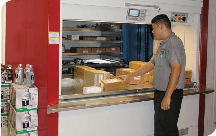
The control screen indicates the quantity to pick and pick lights direct the picker to the exact location of the part.
