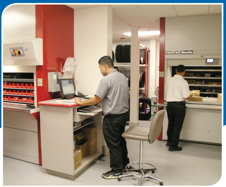
A Kardex Remstar vertical carousel and Shuttle VLM, both almost 24 feet tall, span the facility's two levels maximizing vertical cube space.
