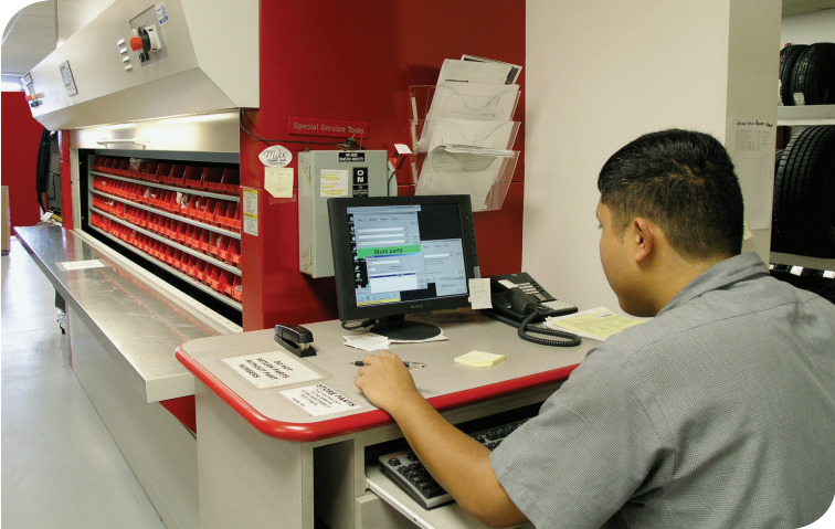
After an order is entered into the Reynolds & Reynolds software an electronic pick ticket is sent to FastPic Auto which organizes the picks for optimized efficiency and positions the equipment for the first pick.
