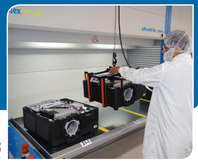
The two Shuttle VLMs were installed with ergonomic hoists to protect all employees and projectors from any potential injury or damage.
