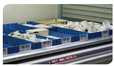
An operator is guided by the TiC to the correct location and they simply pick the part, increasing pick accuracy and productivity.
