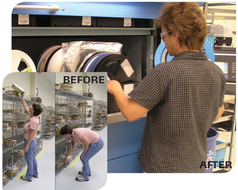
Walking, bending and searching for reels have been eliminated with waist height push of a button delivery.
