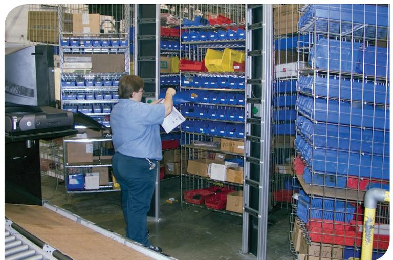
Two Kardex Remstar horizontal carousels to serve as the central distribution point to supply the machine shop and welding workzones.
