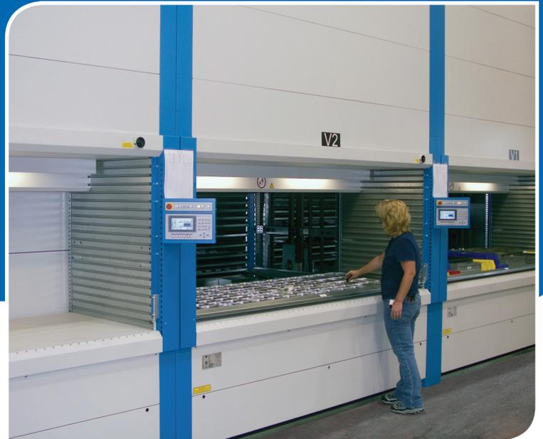
*Using automated storage and retrieval systems with software, Mark Andy has been able to create additional assembly area and manage their parts inventory more efficiently.*
