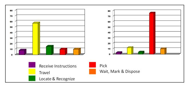
The primary advantage of a vertical carousel is that the system enables the operator to generally remain in a single location, and the carousel delivers the item to the operator. "Commonly referred to as a 'stock-to-operator' system. This removes the walking." In an effort to further reduce travel or dwell time, most industrial facilities opt to implement more than one vertical carousel, known as a "pod."
