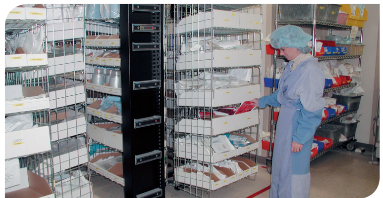
The shelves can have from one to seven cells (or SKU positions) across to accommodate small pieces.
